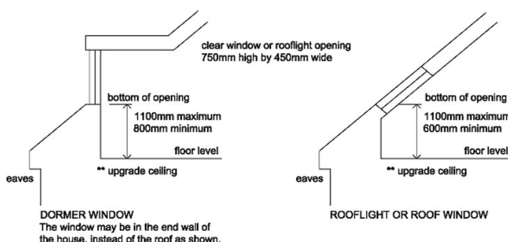
Normally the first floor will require upgrading to achieve a full 30 minutes fire resistance for example two layers of 12.5mm plasterboard with joints staggered.
