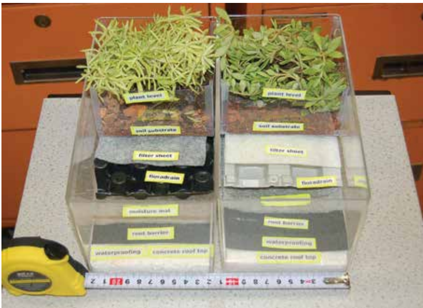
Figure 2.4 Extensive green roof systems from Germany (left) and Japan (right)
